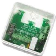
MAK Controller for Energy Saving Application, is a Simple Controller That Works Stand Alone and Control 5A Electrical Circuit, The MAK controller Dirves and accept 2 MEST Sensor with Timer Select: (5Sec - 30 Minutes) and with 2 Logic Allawance: (A= On If Detect Either Sensor Sides, B=On if Detect Sensor1, Off if Detect Sensor2)
