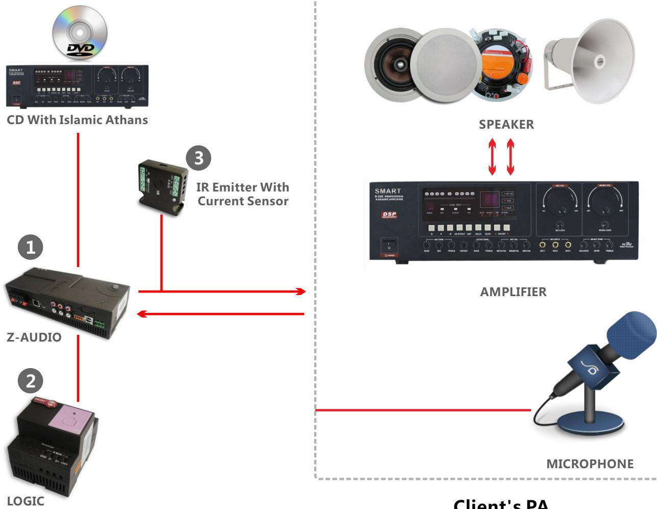
Ingredients: 1 Z-Audio, 1 IR Emitter, 1 Logic Module, 1 Power Supply, 1 CD Player and Prayers CD (Client PA)
