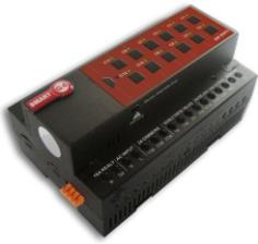
DIN-Rail Mount, Total 3Ch Dimming, and 18 Relays, 1 temp aux, & a 1 VAV 0-10V. To be used as needed with easy assignment for the following applications: lighting, dimming, HVAC, drapes & shutters, boilers or pump, Exhaust fan, Sirens/Flasher, door bell and many more (3ch dimming Each 2Amp / 17ch Relay 5A Each 1 Relay 16A for heavy Appliances), 1 temperature Sensor Input. 1 0-10v output
