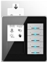
is a wall switch Panel with Easy Print and Slide Labeling Functionality. Built in IR Receiver Plug in Port, (Each Button Enables a different function by pressing left or right), Back lit LED, Double click Macro Function, manual Programming Enabled.
