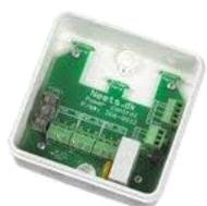
MAK Controller for Energy Saving Application, is a Simple Controller That Works Stand Alone and Control 5A Electrical Circuit, The MAK controller Dirves and accept 2 MEST Sensors with Timer Select: (5Sec - 30 Minutes) and with 2 Logic Allowance: (A= On If Detect Either Sensor Sides, B=On if Detect Sensor1, Off if Detect Sensor2)
