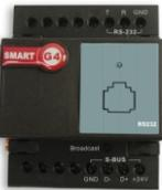
4Ch Dimmer 1A, 20Ch Relay 5A with scene controller. Manual Programming Enabled. (Overload Protection) Good for Lightng Control, 50-60Hz. (Green operated supplied by 24VAC/12mA). Cascadable, Upgradable Via USB Cable. 2-Way status update if manually overridden at Relay side. ((Built in: Added Motor control Double throw Function and Floor heating manual pairing Function))
