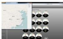
Diesel Engine Monitoring Genset, To monitor and Trigger or dissable Ingition, RPM, Tank, Temp, Power Metering and other. Both RS-232 and IP Enabled with Http. CAN BUS Ready
