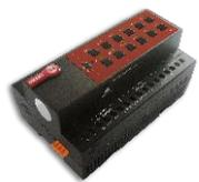
4Ch Dimmer 1A, 20Ch Relay 5A with scene controller. Manual Programming Enabled. (Overload Protection) Good for Lightng Control, 50-60Hz. (Green operated supplied by 24VAC/12mA). Cascadable, Upgradable Via USB Cable. 2-Way status update if manually overridden at Relay side. ((Built in: Added Motor control Double trow Function and Floor heating manual pairing Function))
