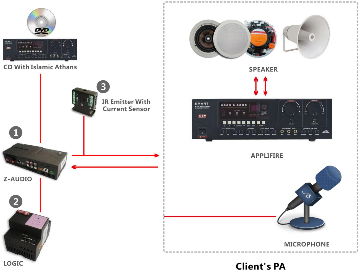
Ingredients: 1 Z-Audio, 1 IR Emitter, 1 Logic Module, 1 Power Supply, 1 CD Player and Athan CD (Client PA)
