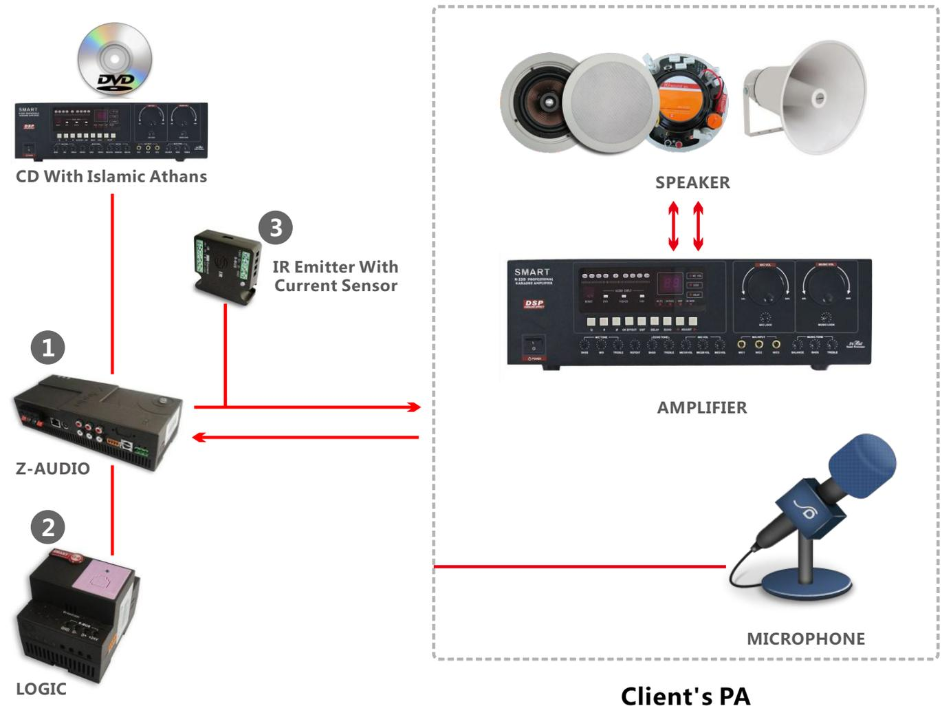
Ingredients: 1 Z-Audio, 1 IR Emitter, 1 Logic Module, 1 Power Supply, 1 CD Player and Prayers CD (Client PA)
