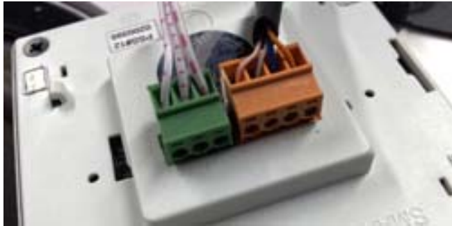
Figure 4 DDP Connected to S-BUS (Orange) and the IR Eye (Green)
