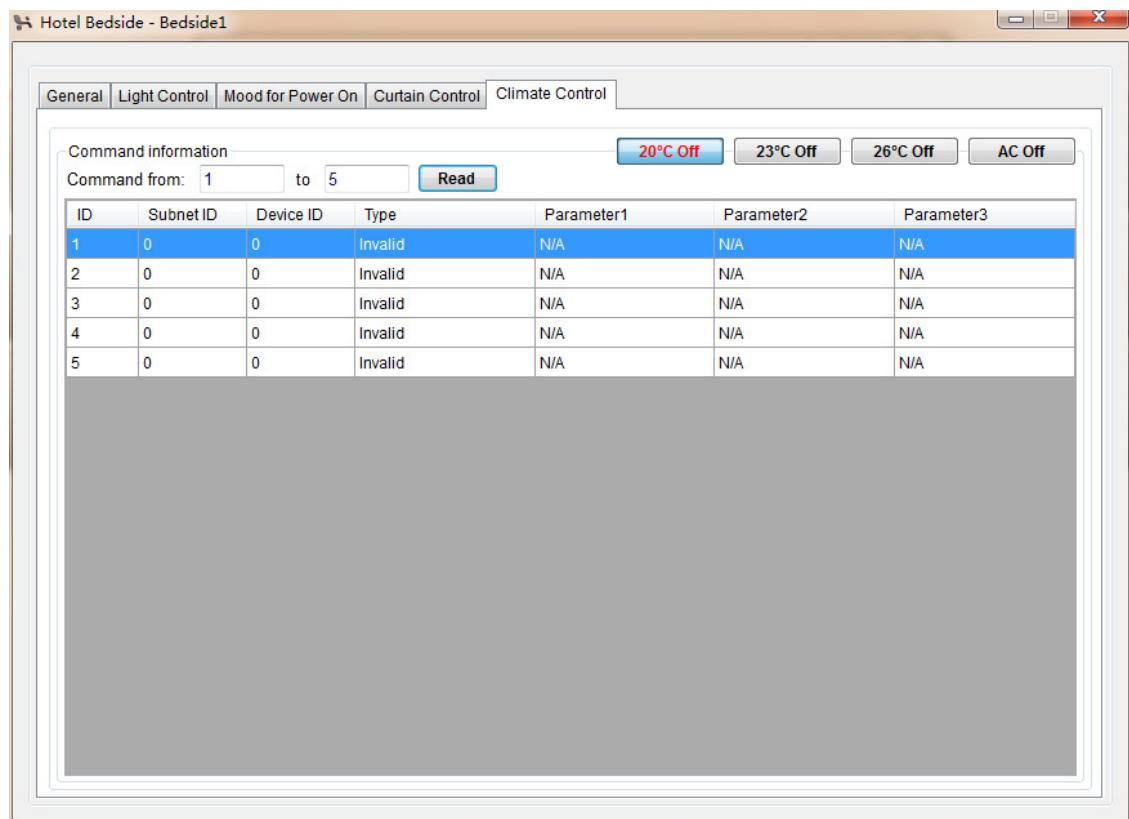
6>Configuration as below: **Notice: The (Switch no.) means the IR Code, and the Parameter 2 must choose the (off) option.**
