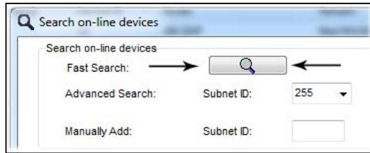
**!** *Fast search can't load all the Network Devices, it is only load part of the devices, it is only good for small project that contain around 10 devices, and to check the network communication with your PC.*
