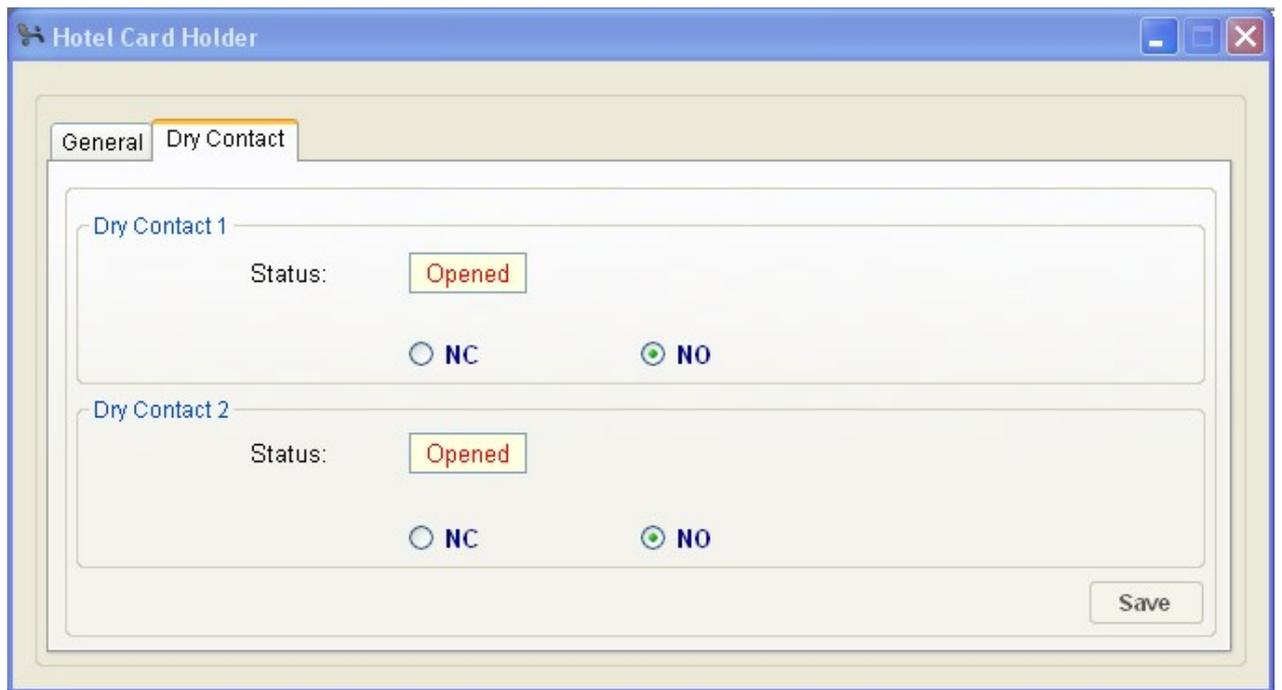
Please know that the dry contact 1 is for external bell, dry contact 1 can connect to normal external bell to turn on /off the bell.
