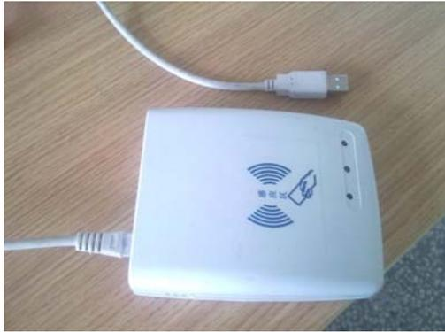
Connect Card encoder device to your computer by USB, it does not request any driver.
