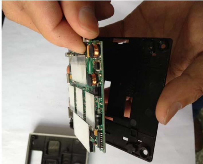
5- At the back cover, push the magnet using the screw driver.
