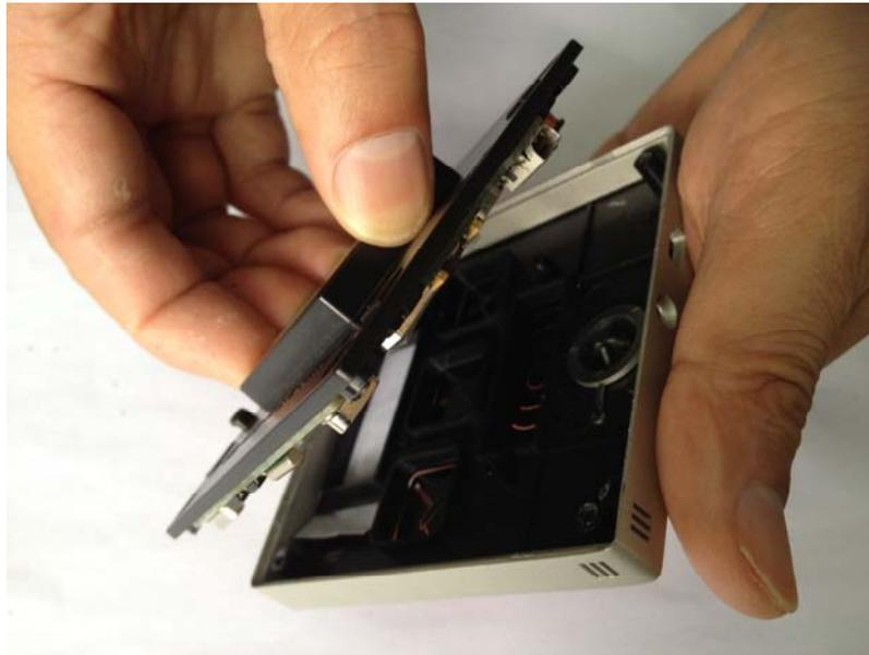
3- Push using screw driver between the PCB and the back cover lock to separate the PCB and the back cover.
