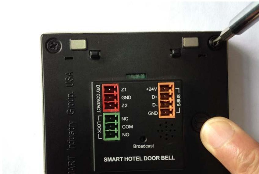
2- Remove the back cover of the Door Bell Panel
