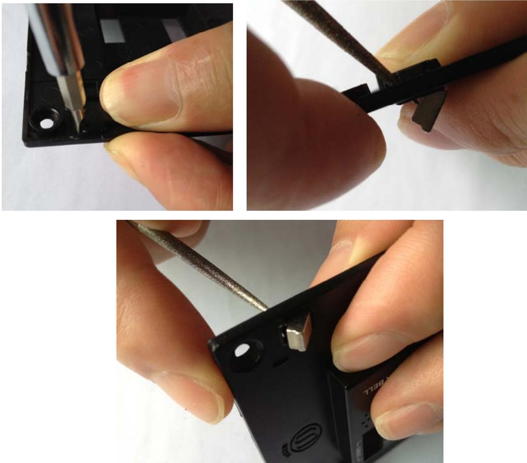
6- Only remove the **one magnet on the corner near to USB Upgrade**, so that it will not make noise.
