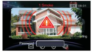
You can see the No. and sensor type in red color showed at the top pf interface. For example: "1:Smoke" to indicate that Zone 1, Smoke sensor is triggered.
