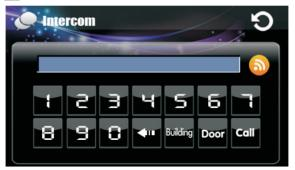
Input 4 digits of Building No. +2 digits of Door No. + 4 digits of Room No., then press **Call** icon to call the resident. For example, if input Building 0001, Door 01, Room 0001, you can input "1" + "Building" + 1 + "Door" + 1, the system will add zero automatically. If input wrong, click **Call** to delete. If the Building No. and Door No. is consistent, you can also input Room No. directly.
