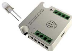
Universal Infra Red code Emitter with built in 2A current sensor and cyclic function. The innovative current sensor Idea check if the electronic equipments is running or is turned off to prevent sending Power Toggling IR code as example. Each module Can save up to 255 IR codes then can be used for Home theater equipment, HVAC, Media systems at living rooms, Curtains control, and several other devices.
