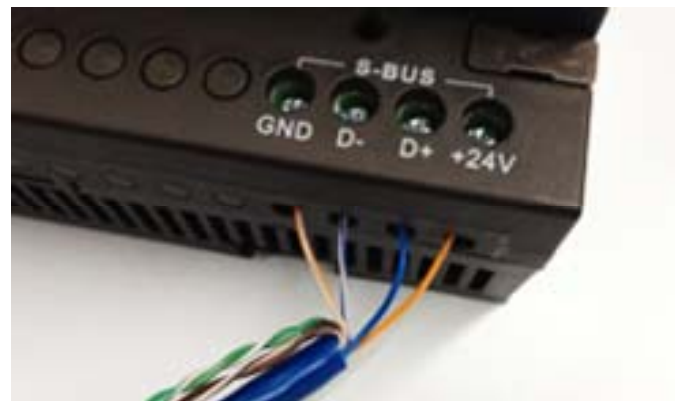
Figure 9 Conventional S-BUS connection
