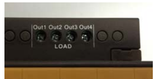
Figure 13 Dimmer's Load output loads.
