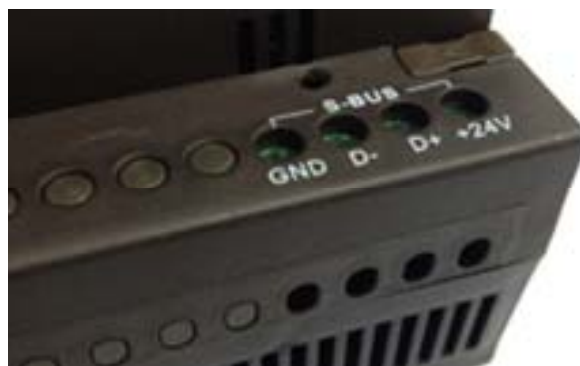
Figure 3 Conventional S-BUS connection
