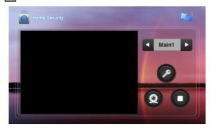
Click Main1 icon to switch into monitoring Main or Sub door panel. Click or icon to select the monitoring object. When select Main 1~9, it monitors outdoor panel; when select Sub 1~9. it monitors the flat panel. Click icon to monitor, click icon to cancel the monitor, click icon to unlock the door.
