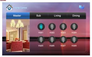
Set the light of corresponding room, such as Master, Sub, Living and Dining (see the room setting for details),8 lights can be set in every room at most. Click the corresponding light icon, then you can control the light turn ON/OFF.
